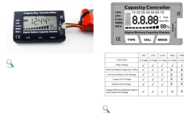
LK Power 2-7S Batteri testare LK2-7S
