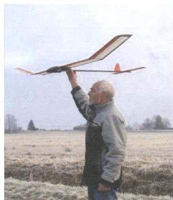
Fig. 2 Skylady in correct attitude for a glide test
