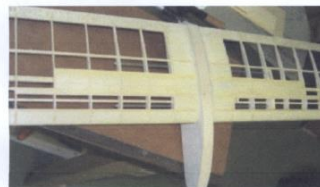
Fig. 8 The wing centre section is shown in greater detail than in Fig. 7. Note the additional spars that reinforce this highly stressed section of the wing.
