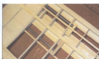
Fig. 9 The underside of the centre section. Note the steel wire joiners passing through ply ribs and the extra spars and balsa sheet let-in between the central ribs.
