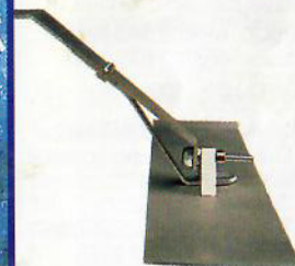
Torsion Bar Bolts to Dural Landing Gear with Supplied Hardware.
