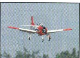
Hal Parenti Competitor F4C Prototype: North American T-28B Trojan Scale: 1:6 Wing span: 2,08 M Engine/s: Moki 1.8 Weight: 10,66 kg.
