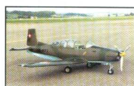
Gody Fischer Competitor F4C Prototype: Pilatus P3-5 Scale: 1:4,5 Wing span: 2,33 M Engine/s: 4-cyl OS Gemini Weight: 10,7 kg.
