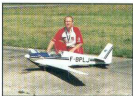
Robert Makowski Competitor F4C Prototype: Fournier RF 4D Scale: 1:3,09 Wing span: 3,635M Engine/s: OS 120 Weight: 8,9 kg.
