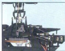
Elevator Push-Pull system Pitch Push-Pull system Servomontage på bom
