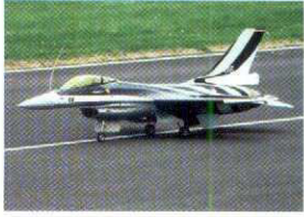
Vitaliy Robertus Competitor F4C/TM F4C Prototype: F-16A Fighting Falcon Scale: 1:6 Wing span: 1,34 M Engine/s: 1 x Jet Cat P-120 Weight: 12,1 kg.
