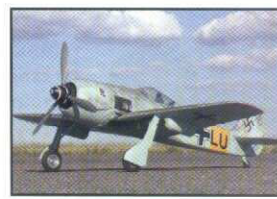
Humphrey Le Grice Competitor F4C Prototype: Focke Wulf 190 A6 Scale: 1:4,5 Wing span: 2,33 M Engine/s: Laser 360 V Four Stroke Twin Cyl. Weight: 13 kg.
