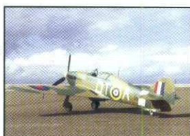
David Knott Competitor F4C Prototype: Hawker Hurricane MK1 Scale: 1:6 Wing span: 2,03 M Engine/s: Laser 120 Four Stroke Weight: 7 kg.
