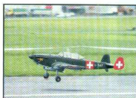
Max Schilt Competitor F4C Prototype: K+W C-3603 Scale: 1:5 Wing span: 2,68 M Engine/s: 2-cyl Four Stroke Patmax Weight: 12,2 kg.
