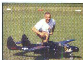
Roger Nieto Competitor F4C Prototype: P61 Black Widow Scale: 1:8 Wing span: 2,5 M Engine/s: OS-91 x 2 Weight: 12 kg.
