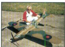
Marian Kazirod Competitor F4B Prototype: Fairey Battle MKII Scale: 1:7,3 Wing span: 2,35 M Engine/s: OS FS-120 S III Weight: 5,9 kg. Reigning World Champion F4B
