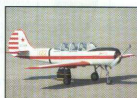
Viatcheslav Chubatov Competitor F4B Prototype: YAK-52 Yakovlev Scale: 1:5 Wing span: 1,83 M Engine/s: OS 20c.c Weight: 5,959 kg.
