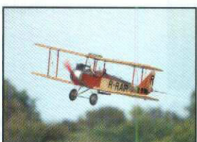
Vladimir Bulatnikov Competitor F4B Prototype: AIR-1 Yakovlev Scale: 1:5 Wing span: 1,76 M Engine/s: Vebra - 61 Weight: 5,7 kg.
