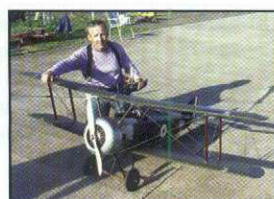
Stefan Olsson Competitor F4C Prototype: Sopwith Pup Scale: 1:4 Wing span: 2 M Engine/s: Laser 180 V-Twin Weight: 8 kg.
