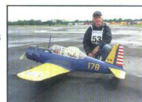
Ulf Jörnheim Competitor F4C Prototype: Vultee Valiant BT13 Scale: 1:5,3 Wing span: 2,4 M Engine/s: Moki 180 Two Stroke Weight: 9,3 kg.
