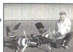
Max Merckenschlager Competitor F4C Prototype: Grumman F7F Tigercat Scale: 1:6,75 Wing span: 2,32 M Engine/s: OS-91 FS x 2 Weight: 10,2 kg.
