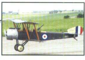
Mick Reeves Competitor F4C Prototype: Sopwith 1½ Strutter Scale: 1:3,3 Wing span: 3,03 M Engine/s: 80 cc V-twin Weight: 13 kg.
