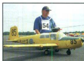
Börje Sebring Competitor F4C Prototype: SAAB Safir C91 Scale: 1:4,2 Wing span: 2,55 M Engine/s: Moki 30 ccm Weight: 10 kg.
