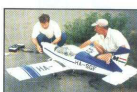
Igor Zhydanov Competitor F4C Prototype: Zlin 142 Scale: 1:4 Wing span: 2,2 M Engine/s: Webra Speed 91 Weight: 7,5 kg.
