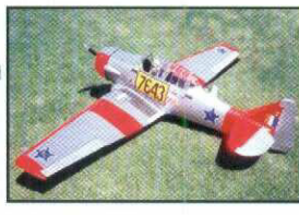
Koos Pretorius Competitor F4C Prototype: North American Harvard Scale: 1:5,3 Wing span: 2,4 M Engine/s: Saito 270 Four Stroke Twin Cyl. Weight: 9,8 kg.
