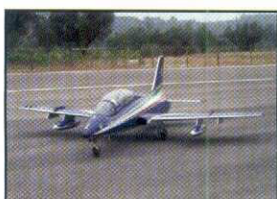
Angelo Minici Competitor F4C Prototype: MB339-A-Pan Scale: 1:5,5 Wing span: 1,9 M Engine/s: Jet Eagle P100 Weight: 12 kg.
