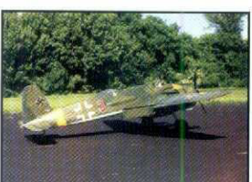
Chuck Snyder Competitor F4B Prototype: Henschel 129 B-2/R-2 Scale: 1:7,67 Wing span: 1,85 M Engine/s: Thunder Tiger x 2 .46 Two Stroke 7,5 ccm Weight: 6,87 kg.
