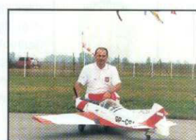
Marek Dabrowski Competitor F4C Prototype: Zlin 526 AFS Scale: 1:4,35 Wing span: 2,035 M Engine/s: OS Max 120 4T Weight: 6,6 kg.
