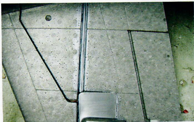
Rund kolfiberbalk ger styv vinge. Skevservo under lock.
