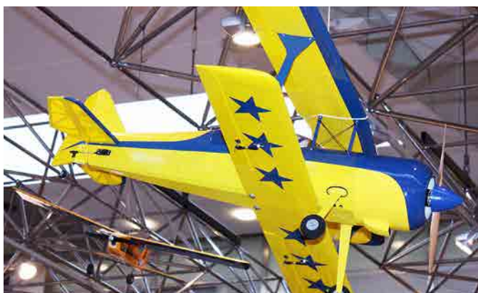
PITS S12 spännvidd 1300 millimeter, elmotor, 6 cells acke. Bo Olofsson.
